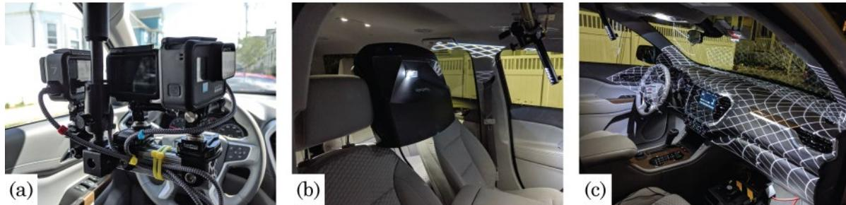
Figure 18. Vehicular system for raw footage capture and carrier signal delivery: (a) the three-view camera mount, (b) the projection system for delivering carrier signal cues and environmental overlays, (c) sample calibration pattern for mapping the vehicle interior
