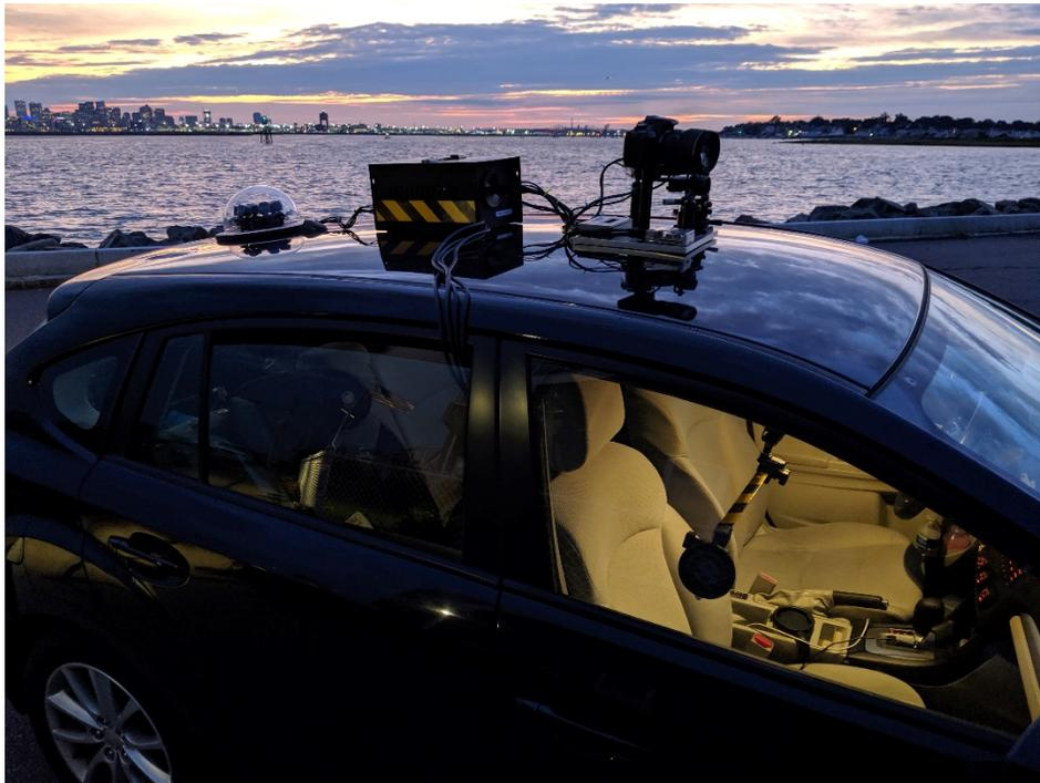
Figure 48. Externally mounted capture and processing system for raw scene data acquisition and initial segmentation.
