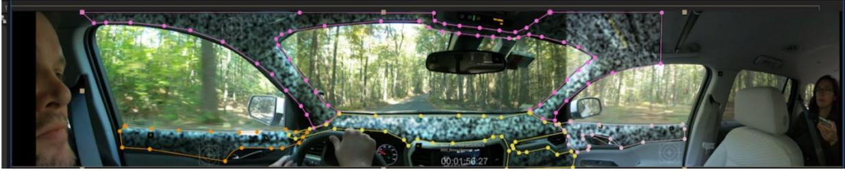
Figure 19. Registration marks for post-processing and stimulus positioning in three-view automotive footage. Full-field overlay shown here demonstrates an example of a projected architecture in the interior of a real-world environment (target: vection augmentation).
